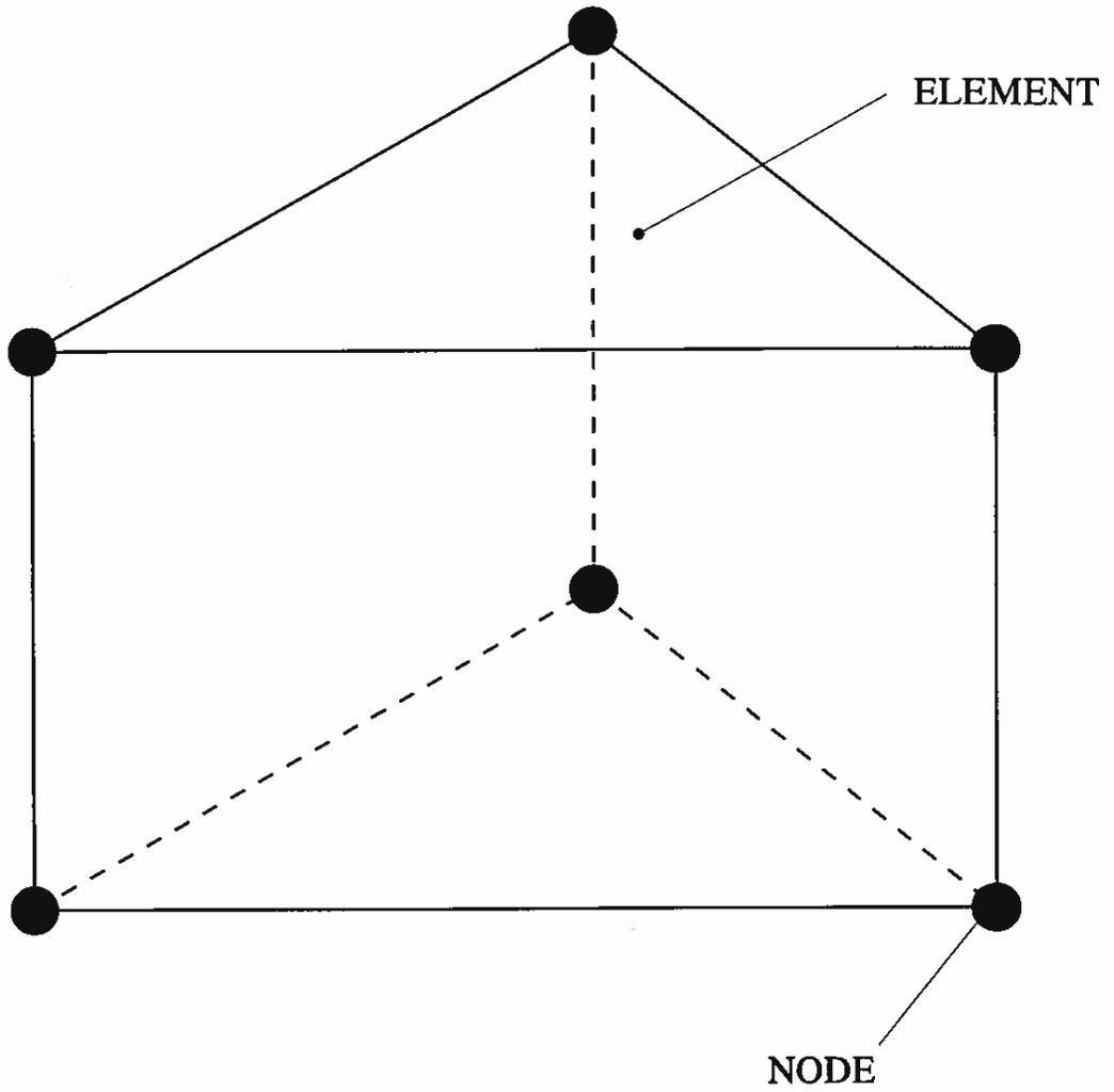
Figure 8-7. Typical element within finite-element mesh.
