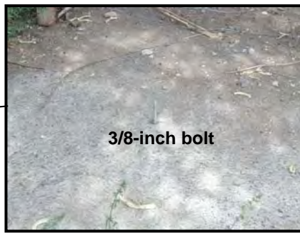
3/8-inch bolt WSBM-13 (1,799.25 ft)
