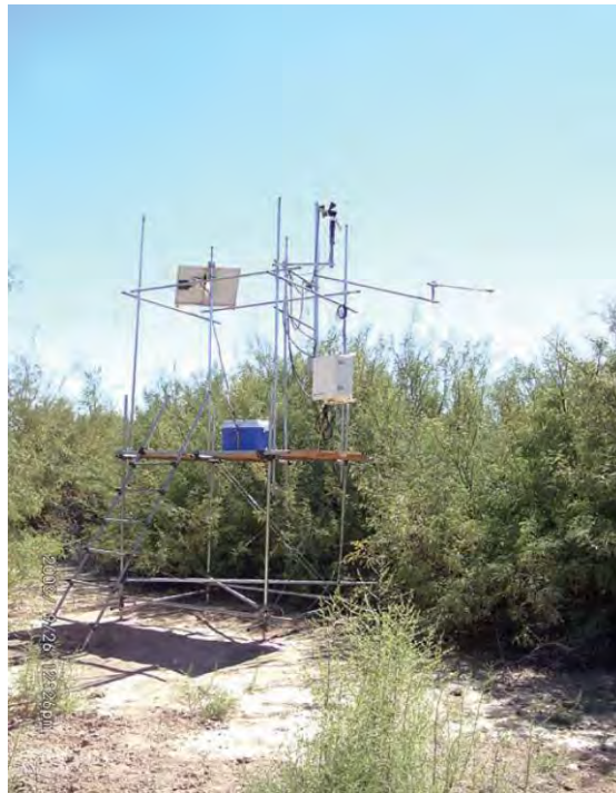
Figure 25. USGS Bowen Ratio Energy Balance station located in the Muddy River area. Modified figure from DeMeo et al. (2008).
