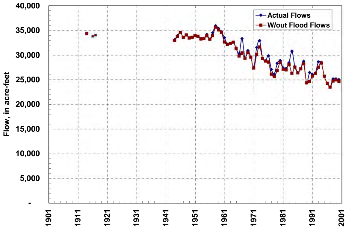
Figure 5-3. Annual flow with and without flood flows at USGS gaging station 09416000 Muddy River near Moapa, NV
