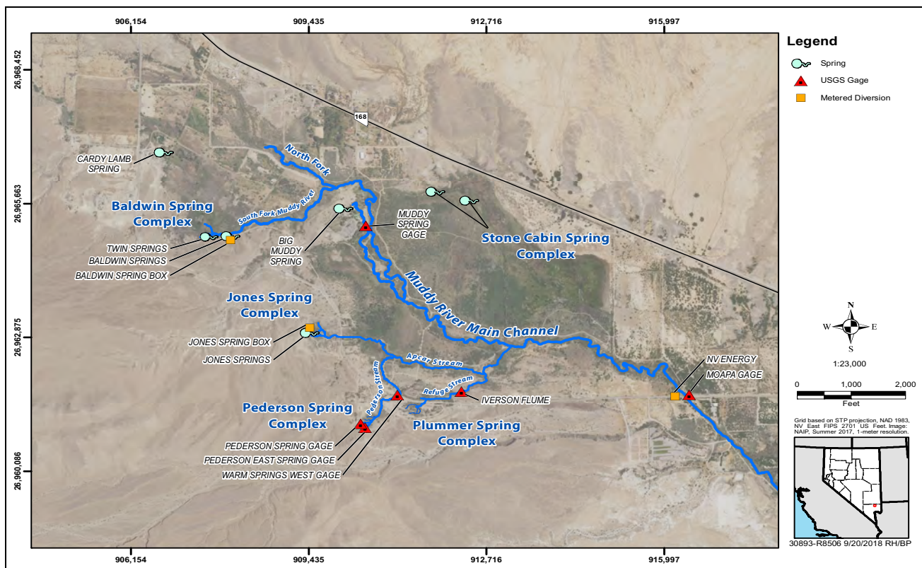
Figure 3-2 Spring Complexes, Streams, Diversions, and Gaging Stations within the Headwaters of the Muddy River
