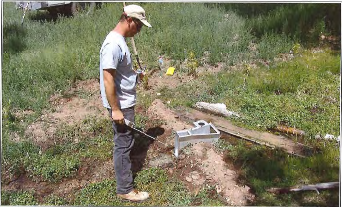
Figure 3-29 Discharge Measurement of Swallow Spring, North Channel, Using a Modified Parshall Flume
