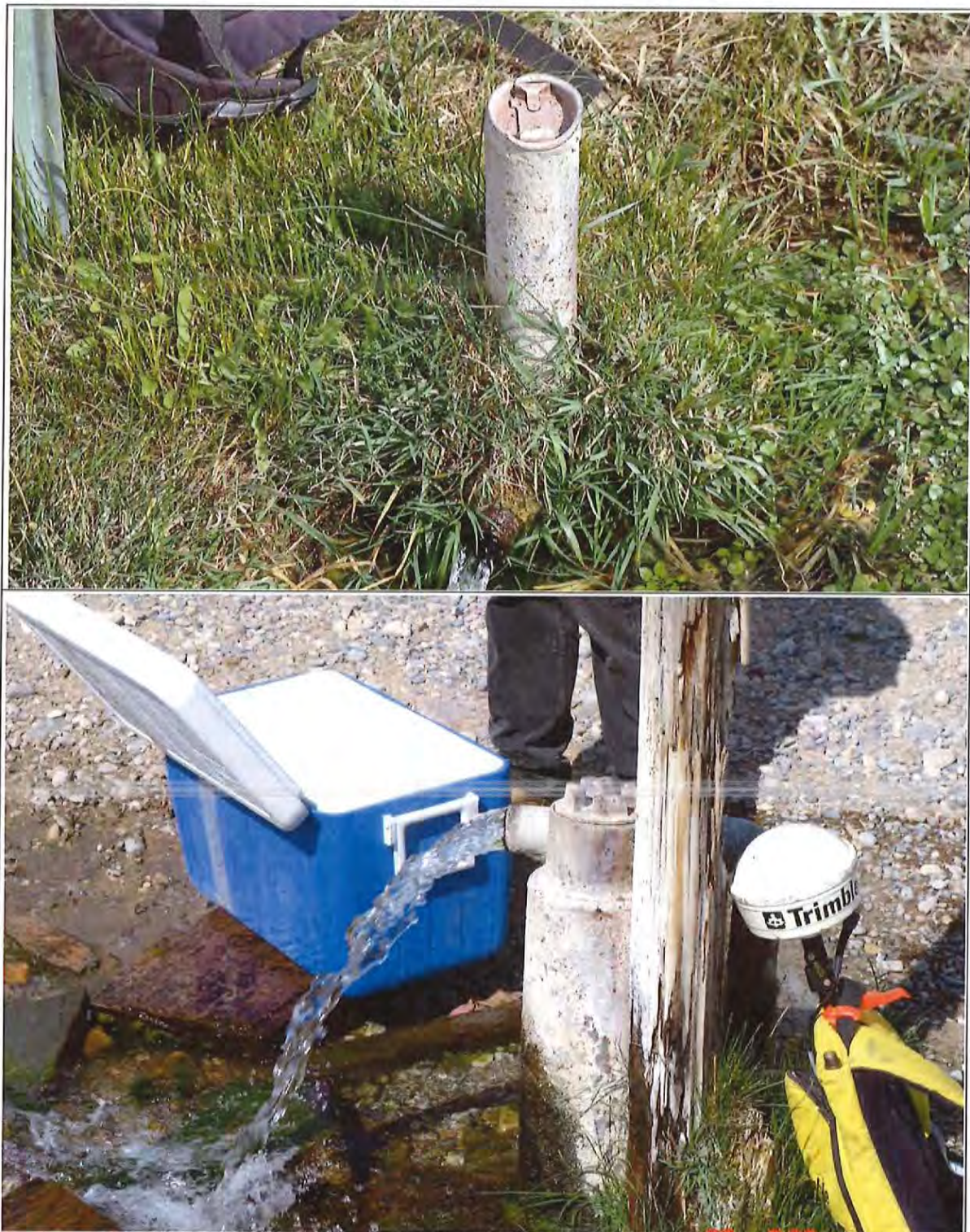
Figure 3-27 (Top) The Cedars #1 is a One-Inch Well, (Bottom) The Cedars #2 is a Four-Inch Well
