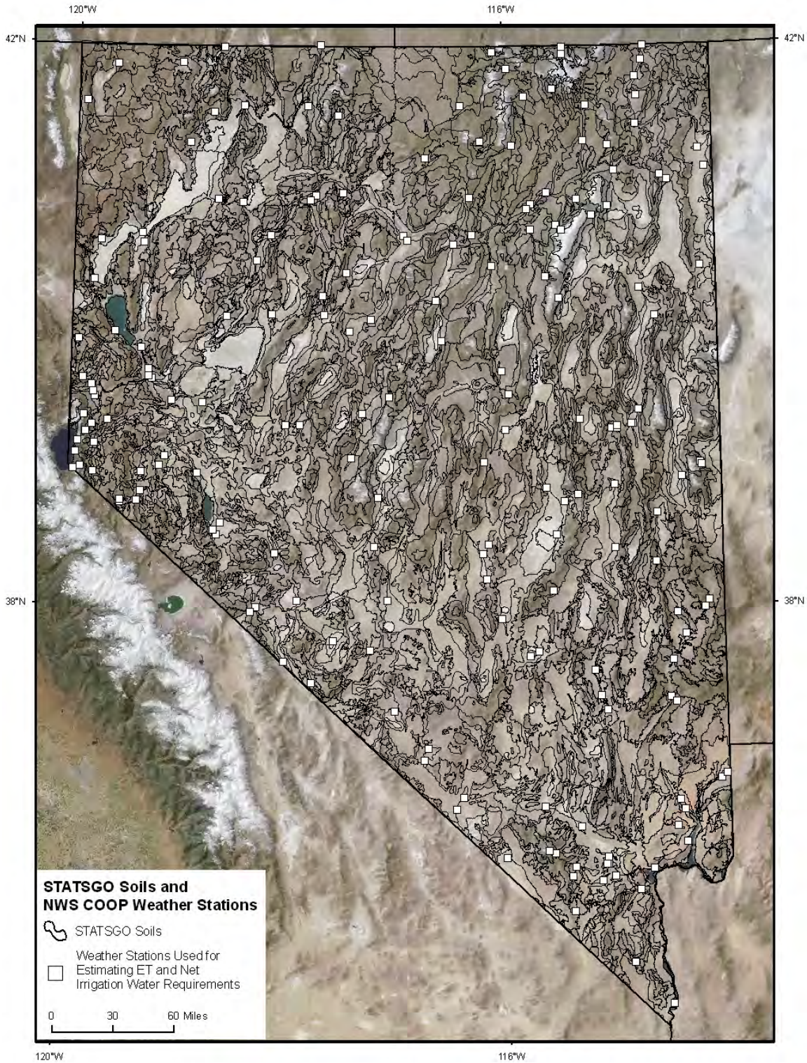
Figure 15. State Soil Geographic Database (STATSGO) used for estimating soil properties at weather stations for soil water balance simulations.
