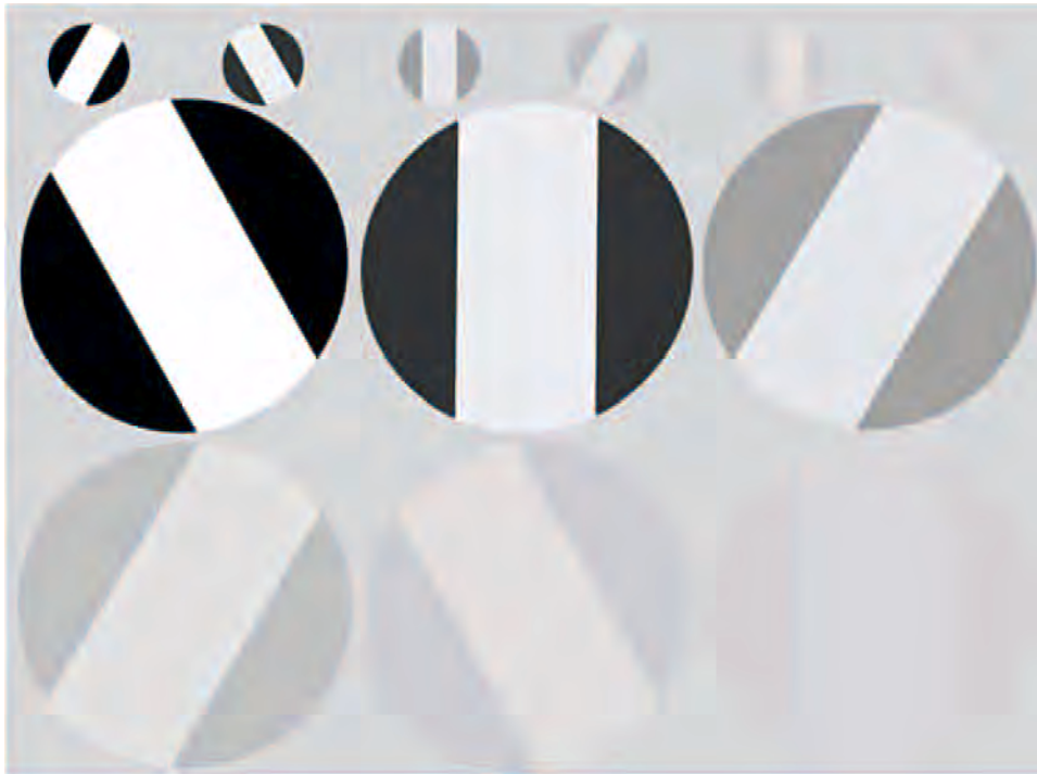
Figure 1. Contrast chart developed by Ayres (1996) and used for matching visibility in conventional photographs.
