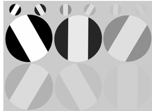
Figure 1. Visual test chart designed to present six contrast levels at each of two spatial frequencies.
