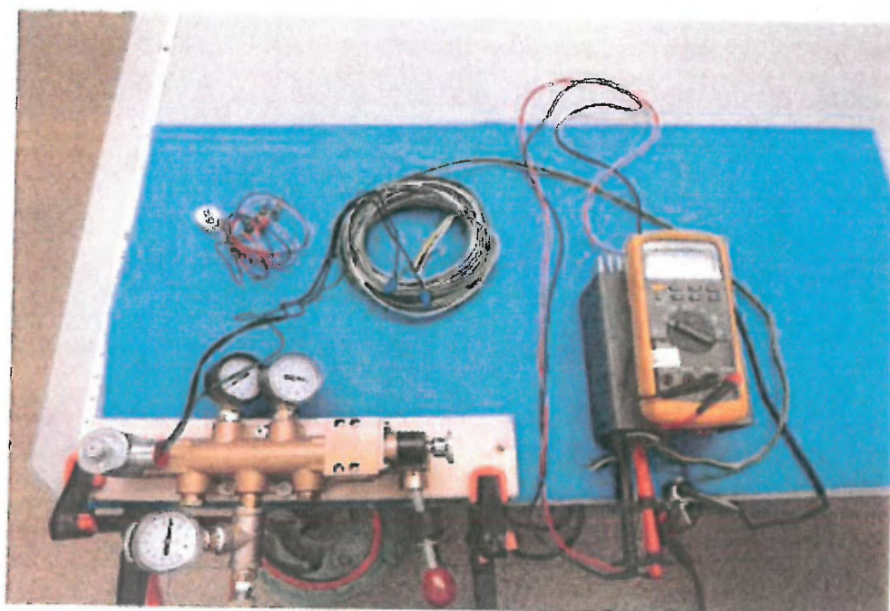
Figure 11-2. Experimental Apparatus for Dump Valve and Control System Testing
