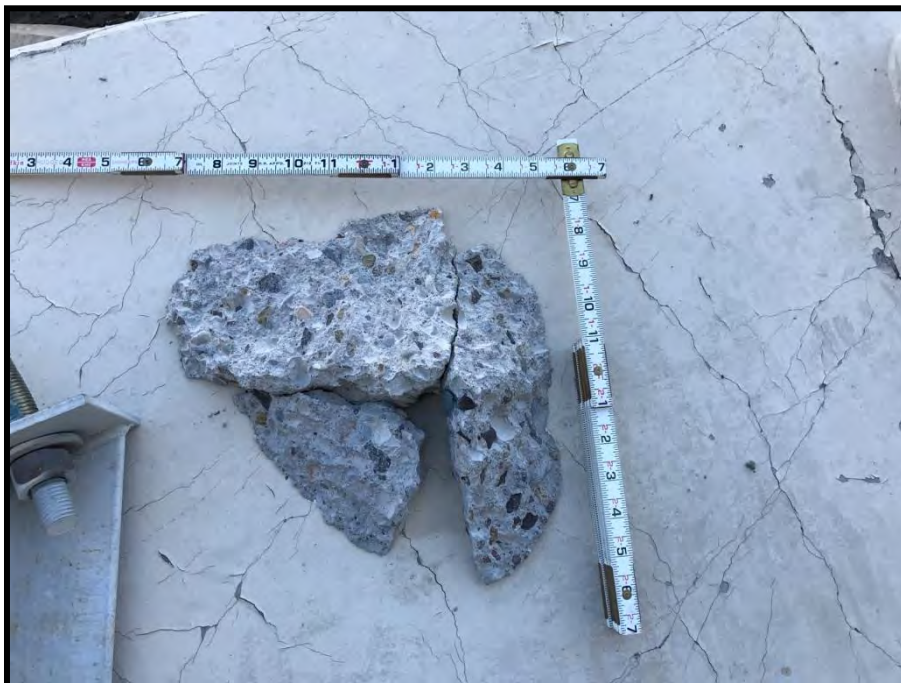
Photo 13: Preserved Failed Concrete at East End Anchor of Spandrel
