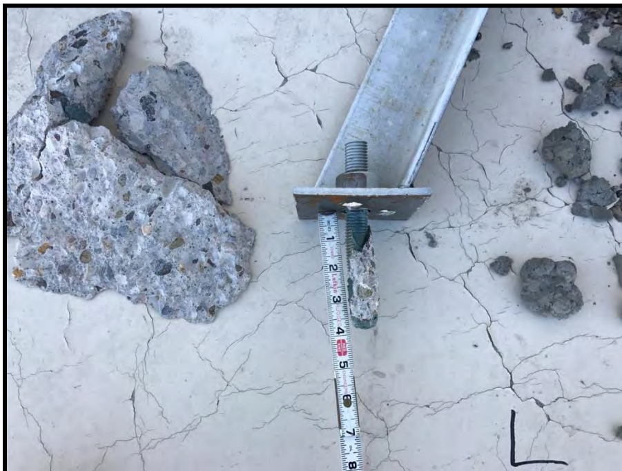
Photo 11: Retrofit Epoxy Anchor Embedment Depth at West End of Spandrel
