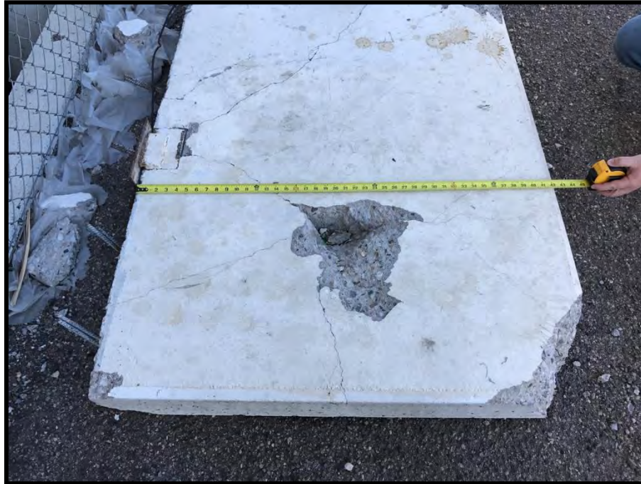
Photo 5: East End Retrofit Anchor Failure Location
