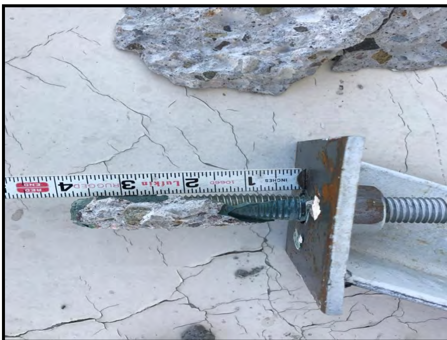
Photo 12: Close-up of Measurement of Retrofit Epoxy Anchor Embedment
