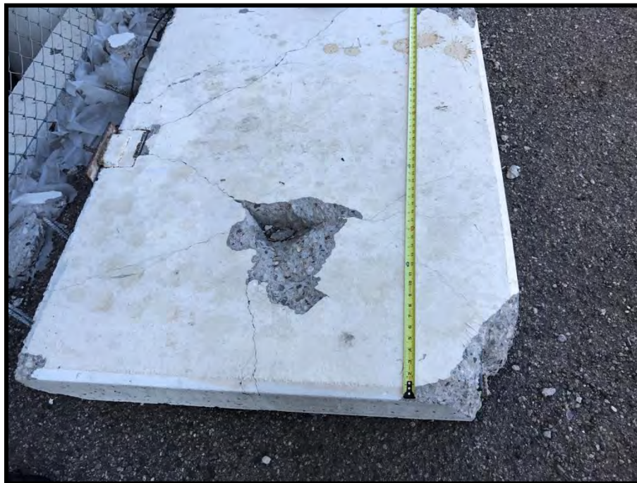
Photo 6: East End Retrofit Anchor Failure Location
