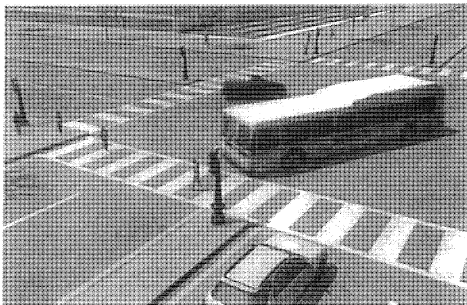
Figure 1-2. Illustration of Collision Type 2—collision between pedestrian and left-turning bus.
