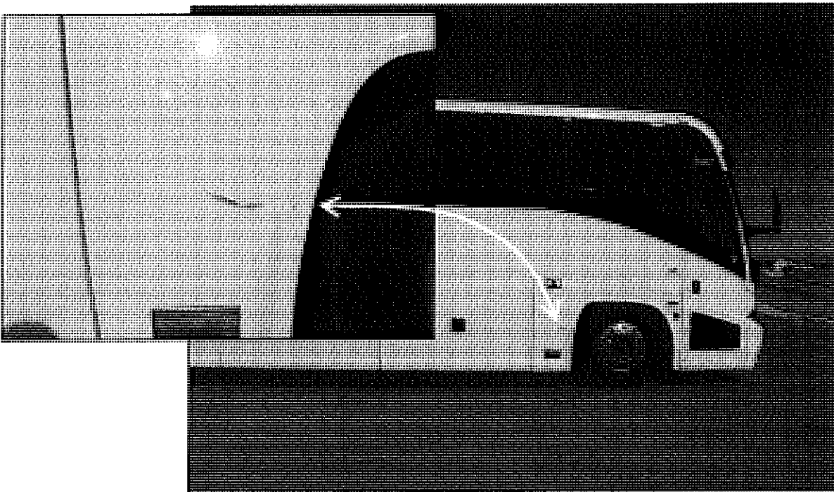
Attachment 3. Contact mark located on the right side of the MCI bus.
