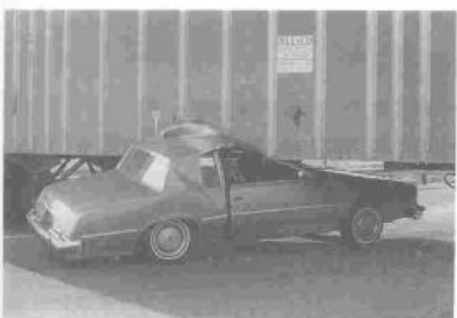
79 Oldsmobile Cutlass Before and After 16 mph (26 kmh) Impact
