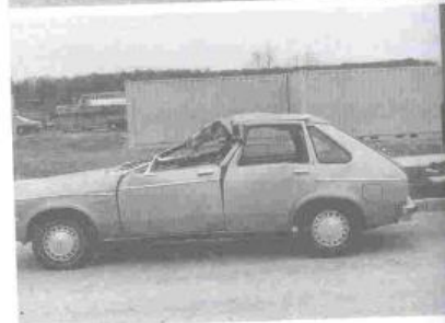
'78 Chevette Before and After 28 mph (45 kmh) Impact
