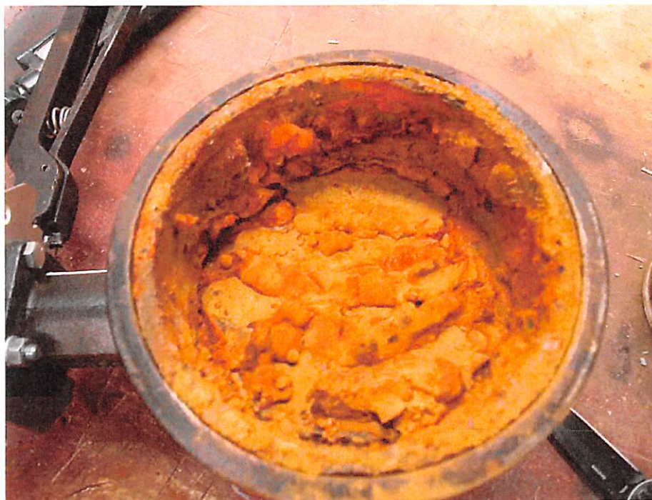
9. BP-2 inlet, outlet, and bypass butterfly valves need to be replaced with stainless steel valves now (jpg31).
