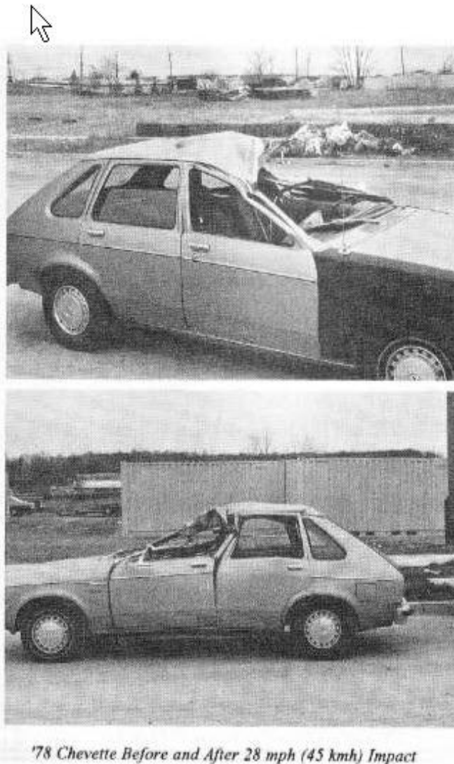
Figure 8: A photograph depicting damages sustained to front pillars, roof and windshield of sustained during a 28 mph crash test where the vehicle came to a stop under a semi-trailer after these structures absorbed the energy of the impact (4)..
