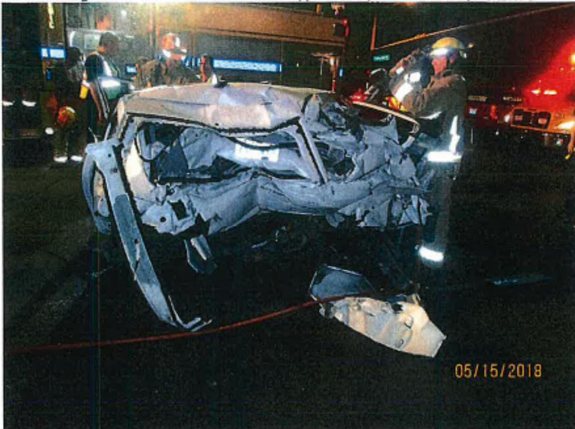
The 2010 Toyota Prius had major damage originating from the rear of the vehicle. The apparent contact damage originated adjacent to the midline of the vehicle, on the driver's side, and extended to the deepest point of crush damage on the passenger side of the vehicle. The above photograph is of the rear of the Prius as rescue personnel was attempting to remove the roof.
