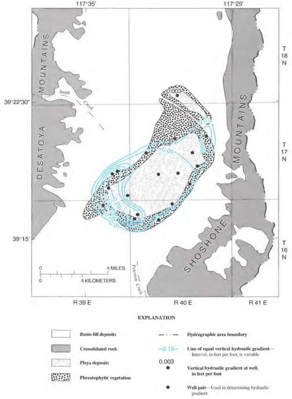
$\label{eq:figure 5.-Upward} Figure 5.-Upward hydraulic gradient in the discharge area of central Smith Creek Valley, Nev.$
