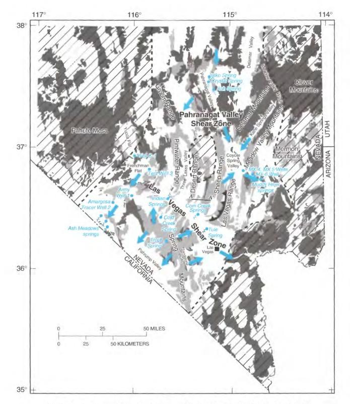
FIGURE 17.—Ground-water flow directions and hydrogeologic features associated with carbonate-rock aquifers in southern Nevada. Modified from Dettinger (1989, figs. 3, 4).
