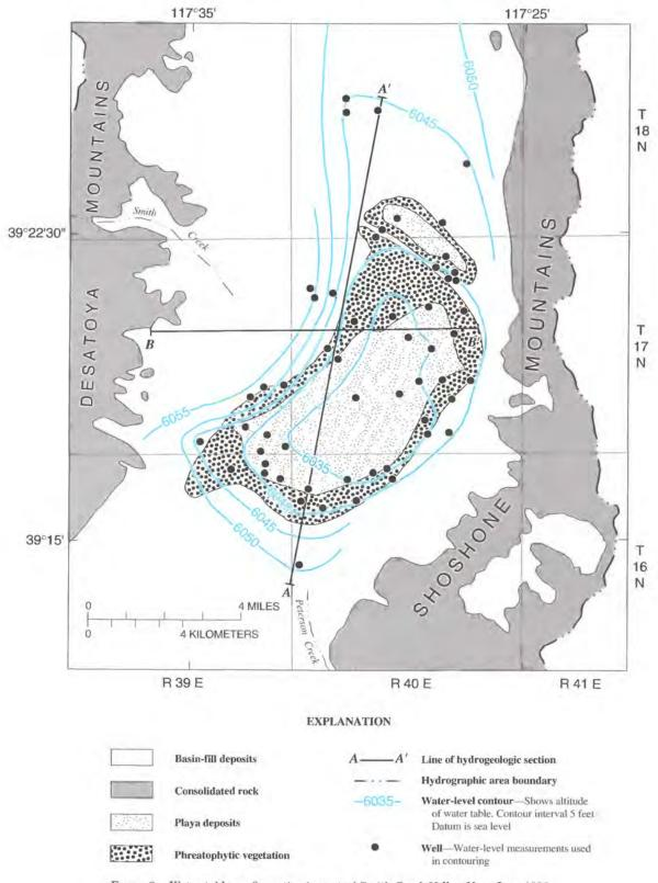
$\label{eq:Figure 3} \begin{array}{c} \mbox{Figure 3.} - \mbox{Water-table configuration in central Smith Creek Valley, Nev., June 1982.} \\ \mbox{Sections $A$-$A'$ and $B$-$B'$ shown in figure 4.} \end{array}$
