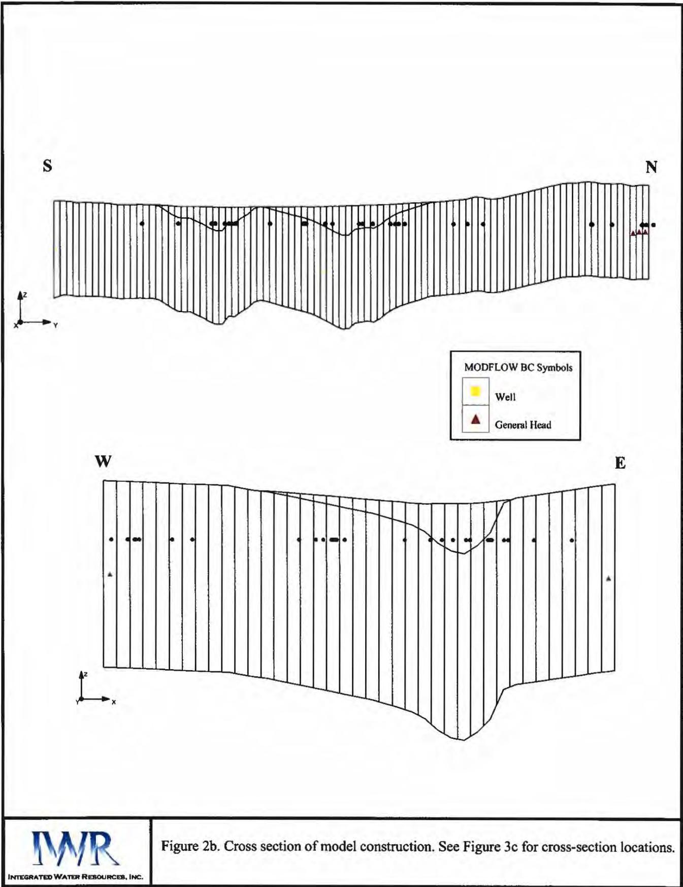
Figure 2b. Cross section of model construction. See Figure 3c for cross-section locations.
